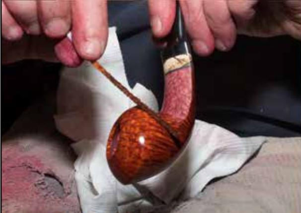
A lot of sandpaper is used, after which it is time to color the pipe. First several layers of a red stain are applied. After that the pipe is polished and sanded again. Then it is time for the final stain, also applied in several layers.
