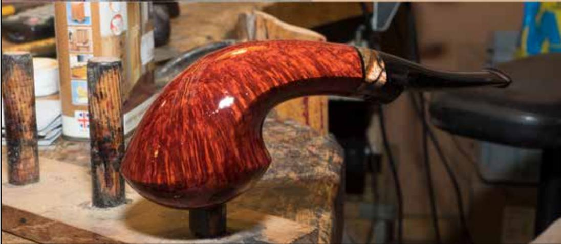
When I was leaving the workshop late in the evening, the pipe was hanging on its stand. It had to dry for at least 24 hours before it could be polished and stamped.
